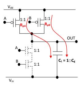
Time taken = tpLH =  $(R_{pA} / / R_{pB}) * C_L$ =  $\frac{1}{2}R_{sp}(1/1) * C_L$ =  $\frac{1}{2}(2.5R_{sn}) * 1 \square C_g$ =  $1.25 \tau$
