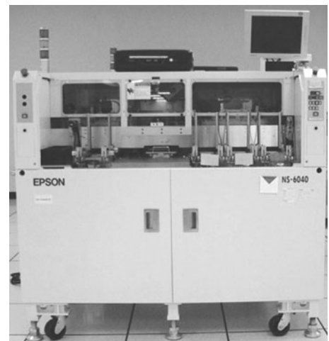
FIGURE 15.5 Photograph of an Epson NS-6040 IC handler (Photo: John Haddy, Cisco Systems.)
