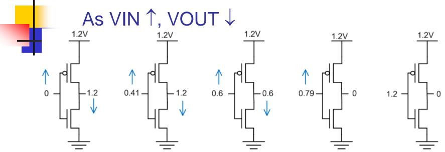
Assume VDD=1.2V, threshold voltage of PMOS and NMOS are 0.4V. |Vthp|=0.4V & Vthn=0.4V. || means magnitude or absolute (don't care about the sign).
