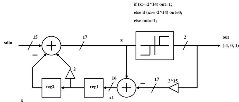
The 2<sup>nd</sup>-order 3-Level Output Sigma-Delta Modulator
