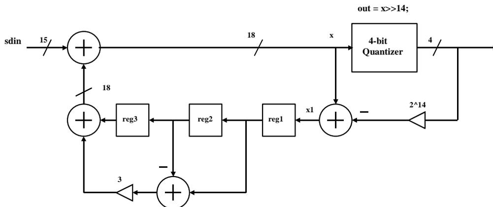
The 3<sup>rd</sup>-order 4-bit Output Sigma-Delta Modulator
